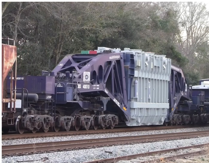
Figure 6. Schnabel car in operation in Theodore, AL on Jan 27, 2013 [54].
